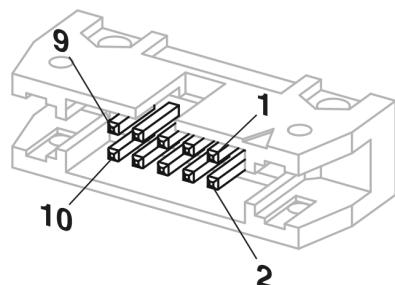
Pin configuration at "Encoder" input:
